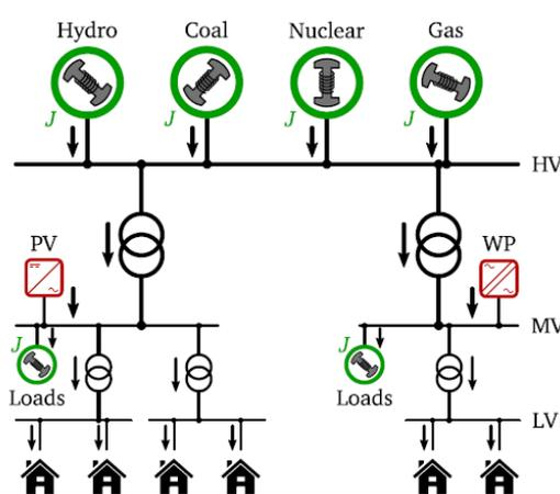
Fig. 1. Traditional structure of the electrical system.
