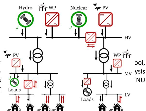
Fig. 2. Electric grid with distributed generation and strong participation of electronic power systems.
